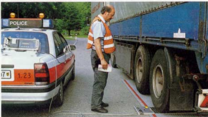
High accuracy WIM systems are now available but legal requirements restrict police to static scales
